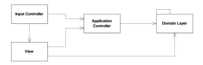
Note that, from the Input Controller's perspective, the Application Controller plays the role of Model in MVC
