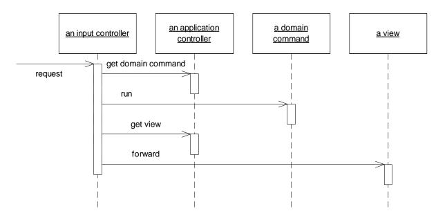
A centralized point for handling screen navigation and flow of an application
